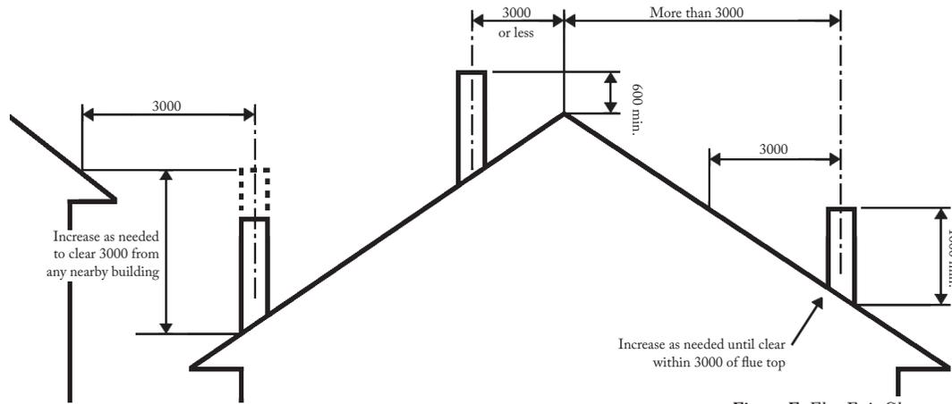
Figure F: Flue Exit Clearances
