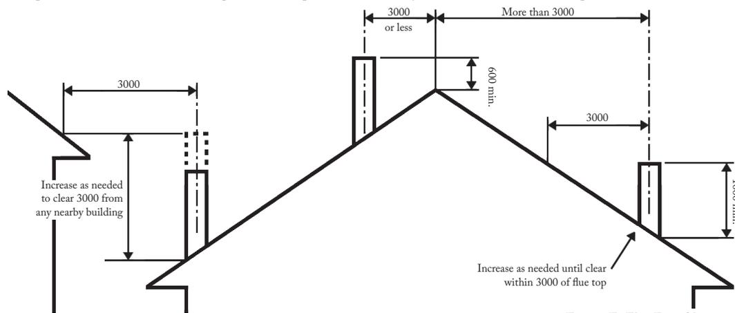
Figure F: Flue Exit Clearances
