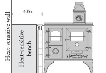
Figure E: Double Shield Example
