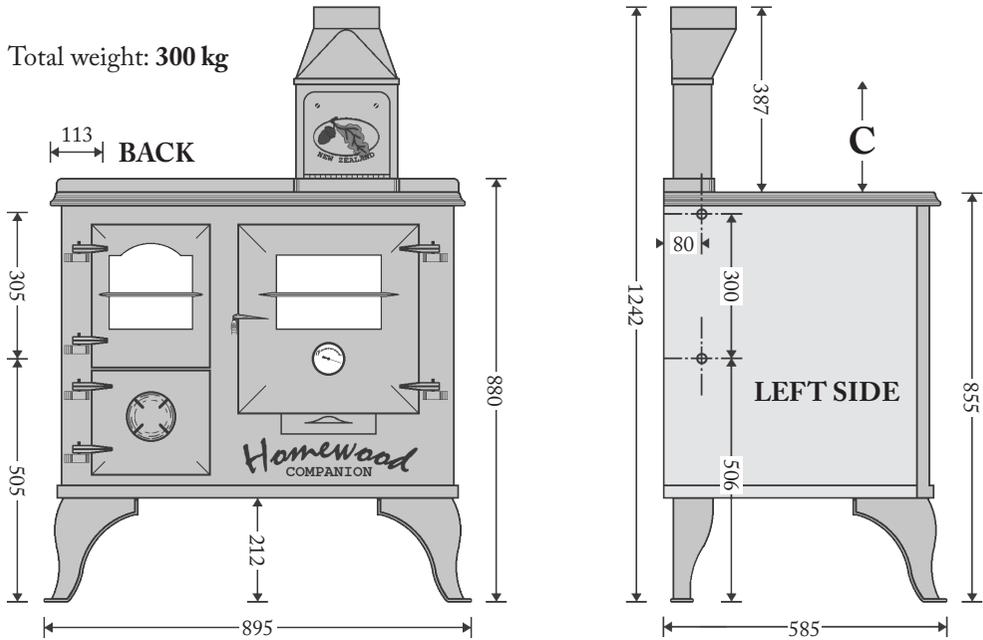
Figure A: Overall Dimensions and Wetback Pipe Locations
