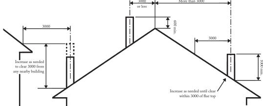
Figure F: Flue Exit Clearances
