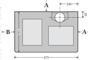
Figure B: Depth, Width, and Flue Collar Location
