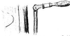
The bypass lever should only ever be in two positions: fully open during start-up, then once your flue has heated up enough to be generating its own draw, fully closed for the rest of the time.
