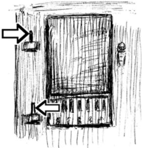
Tapping the pins in the directions indicated will *tighten* the firebox catch. To *loosen* the catch, reverse the tapping directions. Most adjustments should require moving only the top pin. While changes to the ash and left oven doors will be identical to this, the adjustments for the right oven doors will be opposite.
